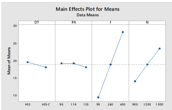
Figure 2: Main Effect Plot for Means of MRR
